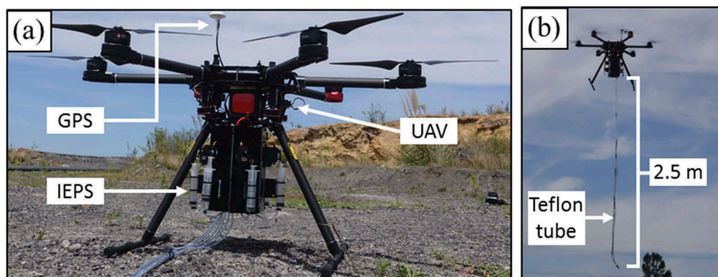
Figure 5. Remote water sampling system integrated onto a UAV: (a) on ground and (b) in flight.
